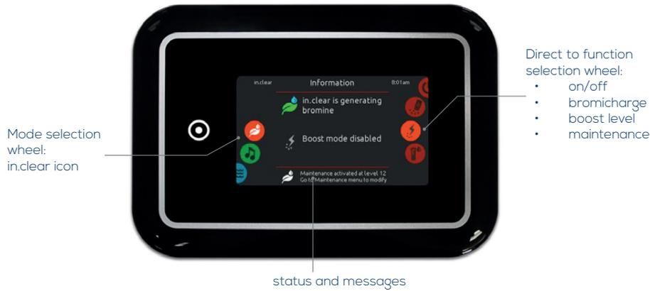
To select the sanitization mode, slide the left wheel up or down until the in.clear icon menu is highlighted in the middle.
