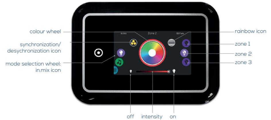
To select the colour mode, slide the left wheel up or down until the in.mix icon menu is highlighted in the middle.
