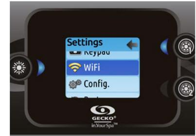
After a few seconds the available networks will appear on the screen, as well as their signal strength. Use the Up/Down keys to move through the list. Select your network by pressing on Light key. If the WiFi network is password protected enter it when prompted.
