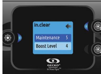
Press on the Mode key to access your in.clear module. This menu allows you to activate or deactivate your in.clear, to start or stop a Boost, and to enter diagnostic mode.
